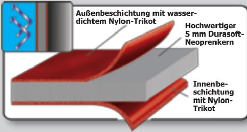
**LIQUID SEAM PROTECTION (LSP) TECHNOLOGIE**
